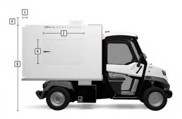
Refrigerated box available in two dimensions, certificated refrigeration unit placed on the roof and remote control with LCD in the cab. Operating temperature:  $0^{\circ}\text{C}$  / +4°C. Compatible with ATX range N1 road approval.
